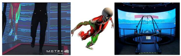
On the left, real-time motion acquisition and coupled biomechanical model visualisation; at the centre 3D visualisation of the Motek's Human Body Model (HBM) and on the right one of Motek's Computer Assisted Rehabilitation ENviroment (CAREN) systems, consisting of an instrumented treadmill, mounted on a motion platform, surrounded by a motion-capture system with giant wrap-around projection screen, all driven by the in-house D-Flow software.
